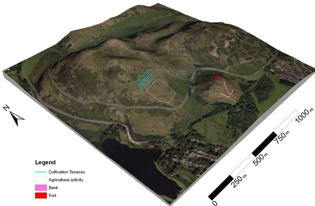
Figure 12. Survey data overlaid onto the DTM with a google satellite image draped ontop.
